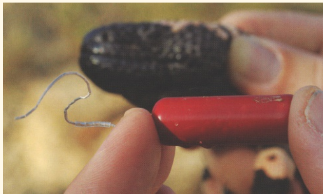
The radio transmitters like this one that scientists surgically implant into Gila monsters are about the size of an AA battery. A radio collar wouldn't work because it would get in a Gila monster's way as it squeezed under rocks or into holes.
